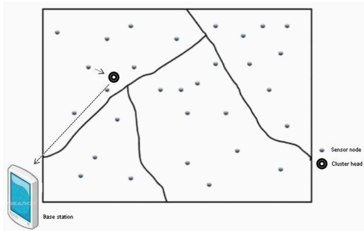
Figure 2. A typical cluster-based wireless sensor network scenario
