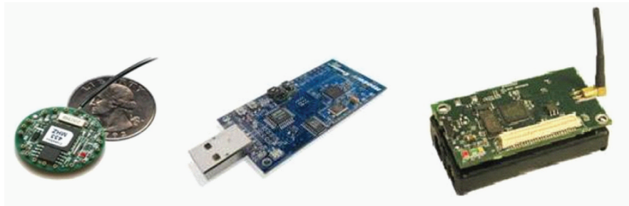
Figure 1. Sensor nodes of WSN. (Source: Crossbow Inc. [left & right], Sentilla Corp. [middle])
